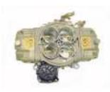
Vacuum secondary version of 800 aerosol billet. Secondary's have a pneumatic Jet System and Quick Change spring kit to adjust power for Slick Track or limited tires. Great for IMCA or Wissota Modified.
