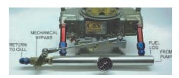
4515-S Dual Pressure Bypass- Methanol
